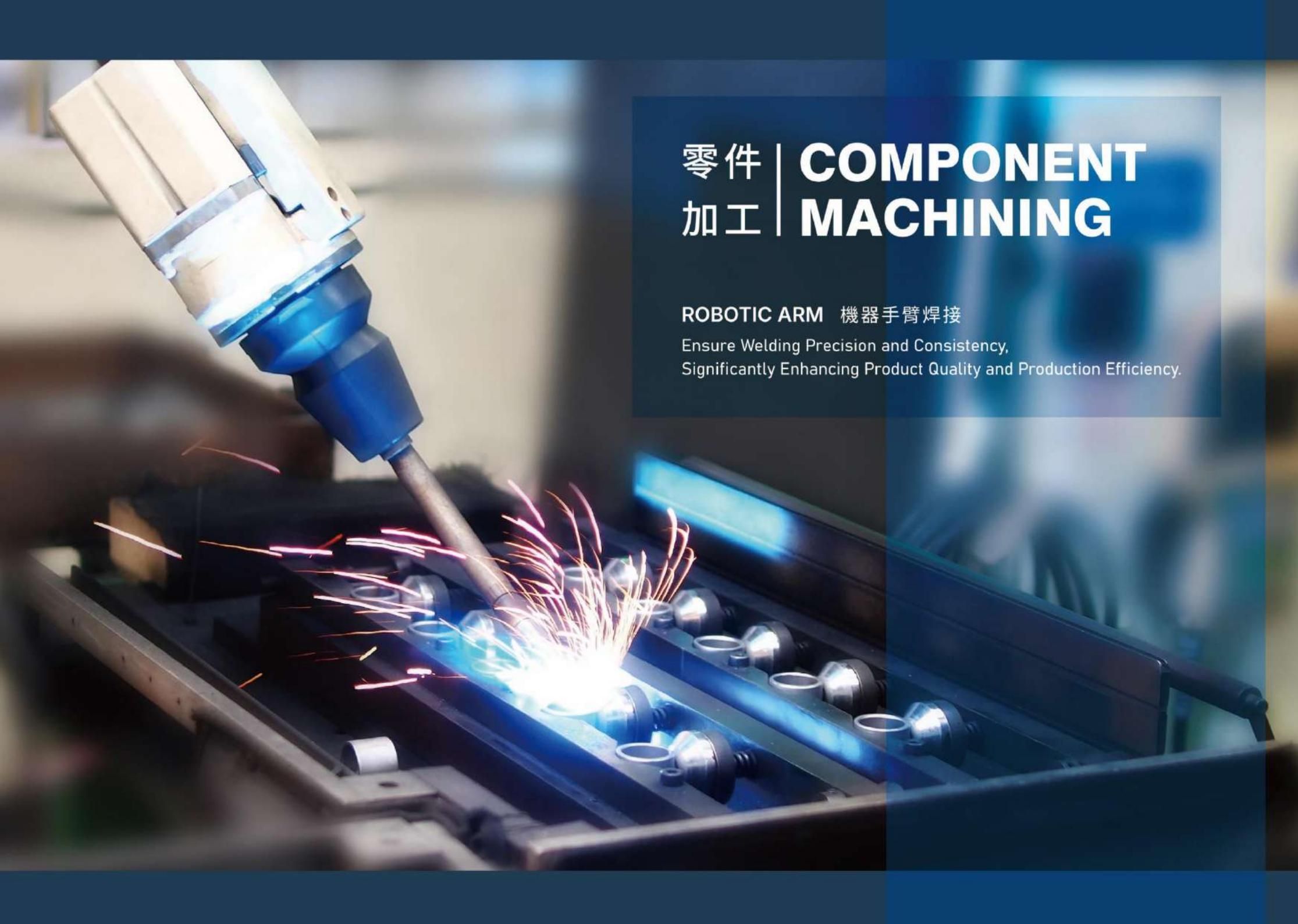
A close-up photograph of a robotic arm's welding torch in action. The torch is blue and white, and it is emitting a bright blue light and numerous sparks as it welds a metal part. The background is dark and out of focus, showing more of the industrial welding setup.
